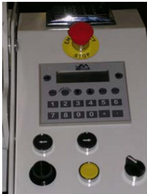
Typical operator display XBT-R400 and controls /
