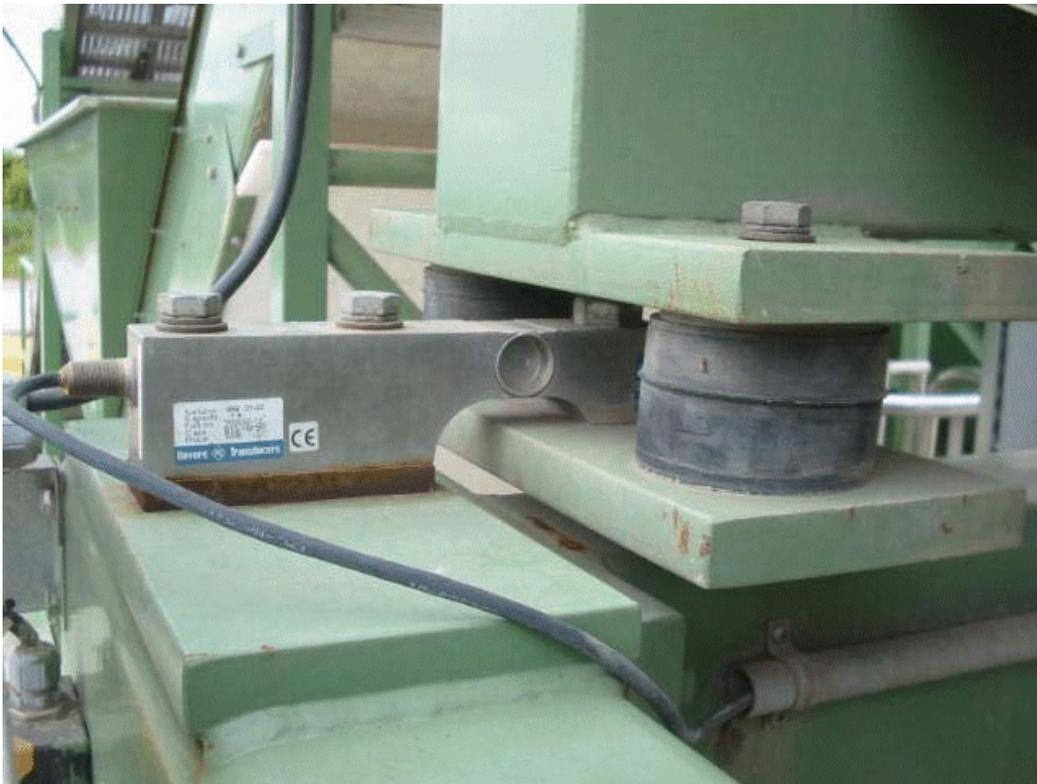
**Typical load cell mounting / Support typique des cellules de pesage**
