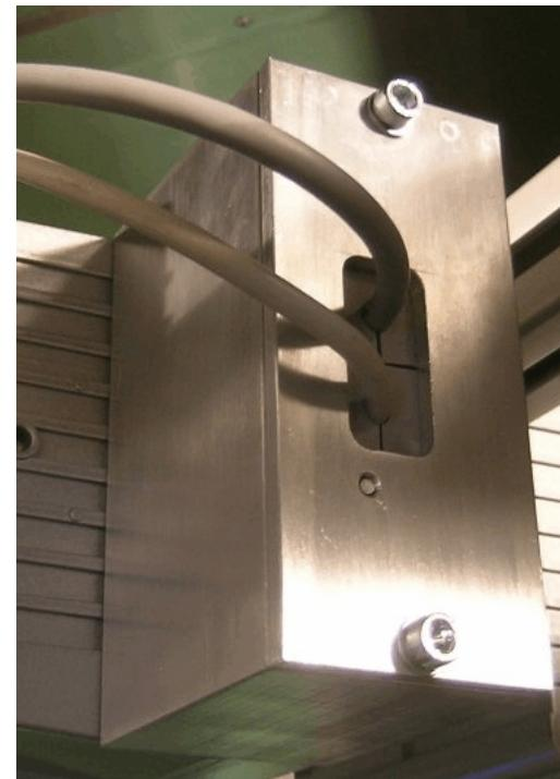
Connector sealing on dimensioning head /
