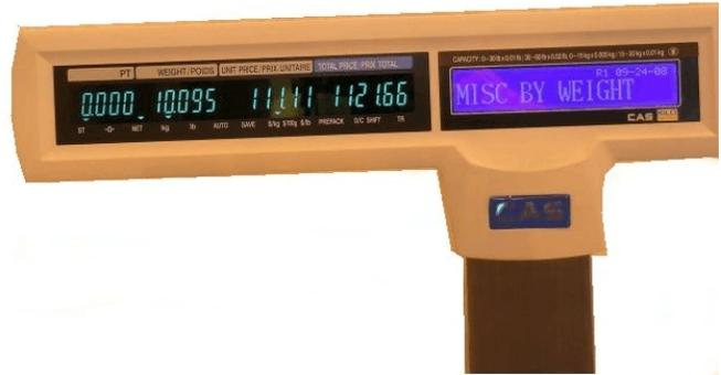
**Typical VFD operator or customer display
