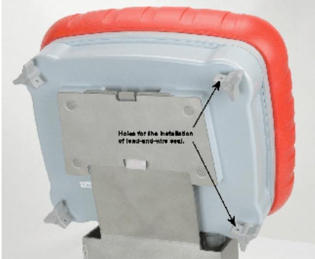
**Sealing method for Infiniti model /
