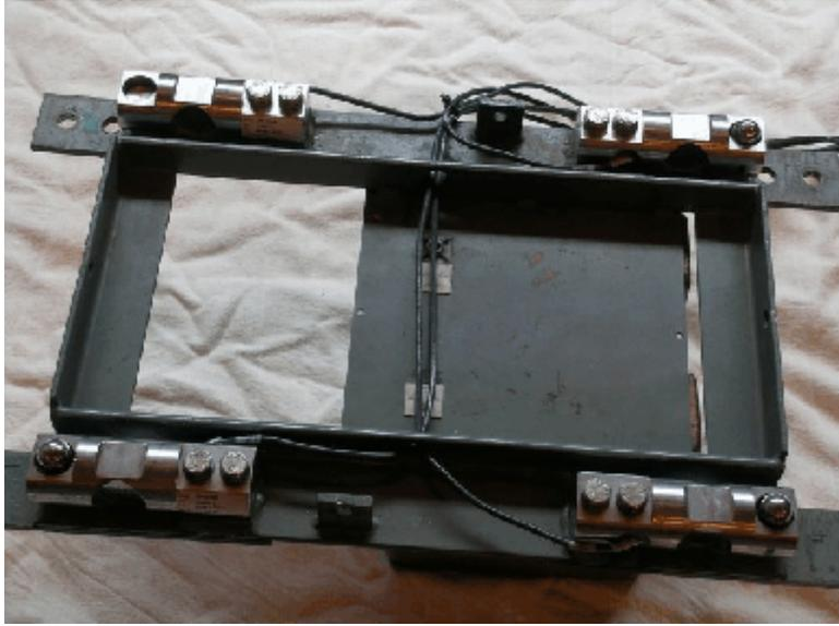
**Typical Frame with Load Cells/
