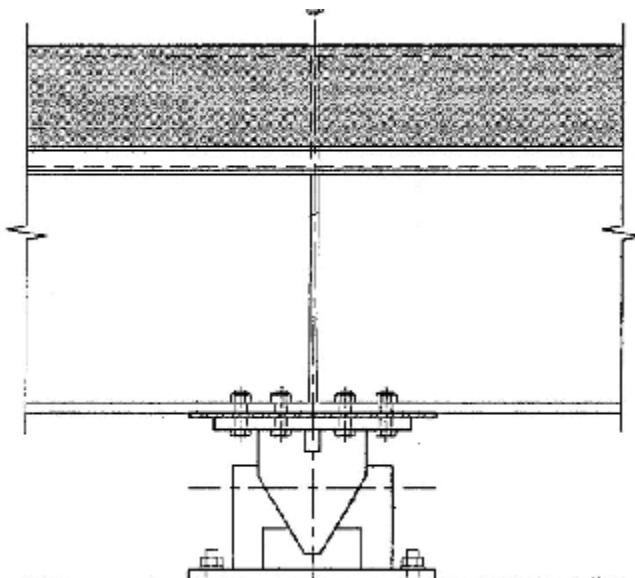
**Side view of load cell mounting /
