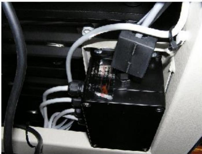
**Sealing of Junction Box with Paper Seal for CubiScan 150-
