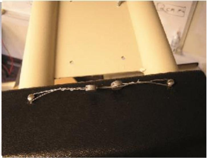
**Sealing of Height Sensor for CubiScan 150-LFT /
