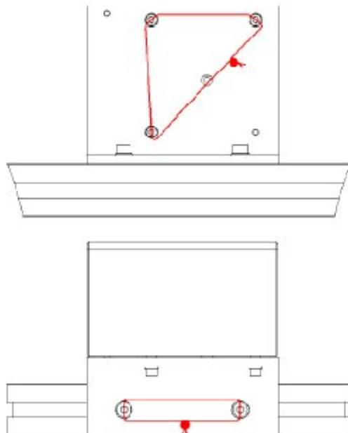
**Sealing of measuring head to frame /**
