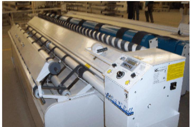
**Typical Cut'n Roll Device/Cut'n Roll type**
