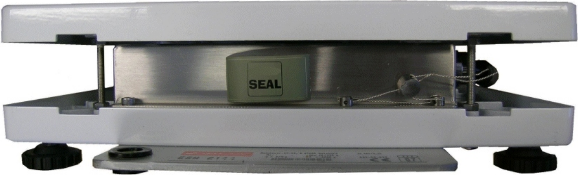
Typical Sealing / Scellage typique
