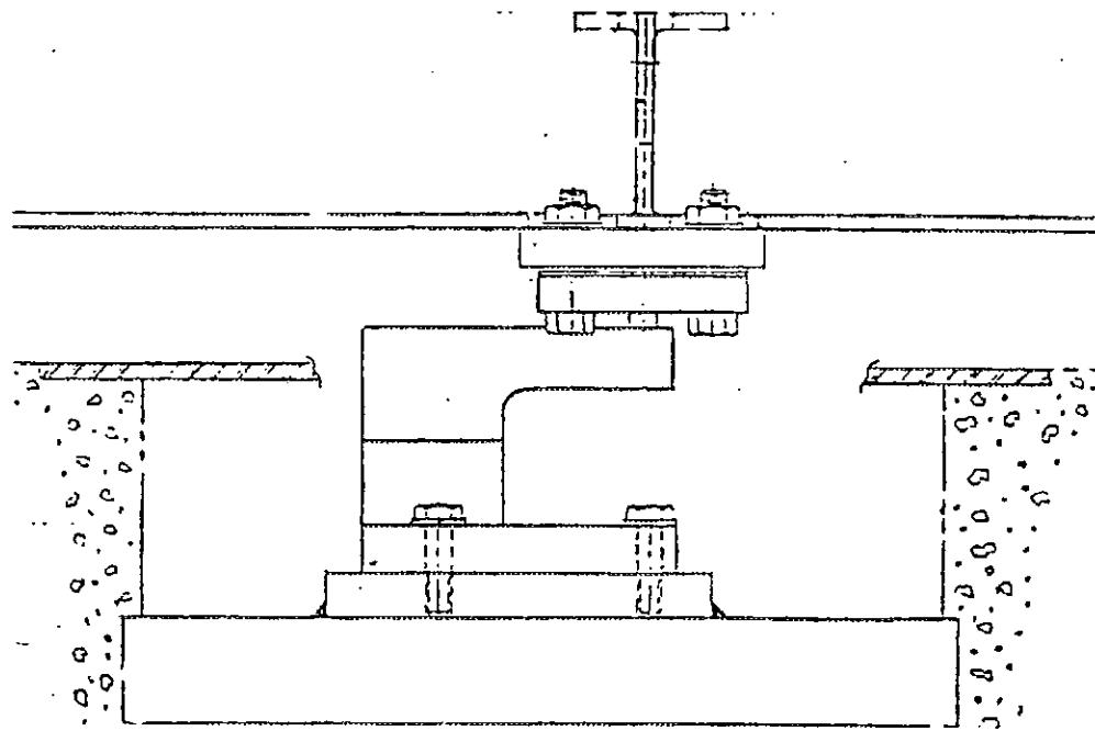
**LOAD CELL MOUNTING/MONTAGE DE CELLULE DE PESAGE**
