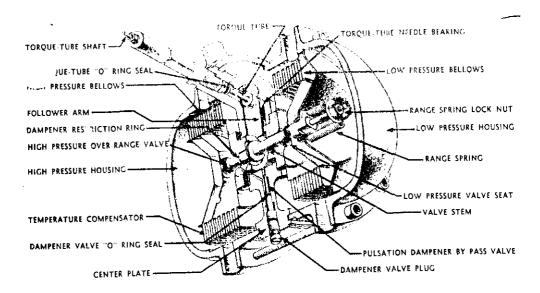
The range of the unit may be simply changed by changing the range spring assembly on the end of the bellows valve stem.
