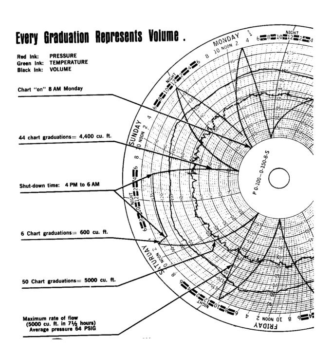
The conventional outer edge scallop models and the full scallop chart recorders perform basically the same function, but the volume record in the latter is presented across the full span of the chart and thus can provide an easy to read record of the metered volume. (see attached facsimile)
