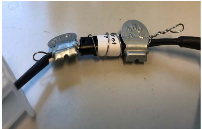
Figure 4 & 5: Typical sealing of the interchangeable Wiegand sensor assembly / Scellage typique de l'ensemble capteur Wiegand interchangeable.
