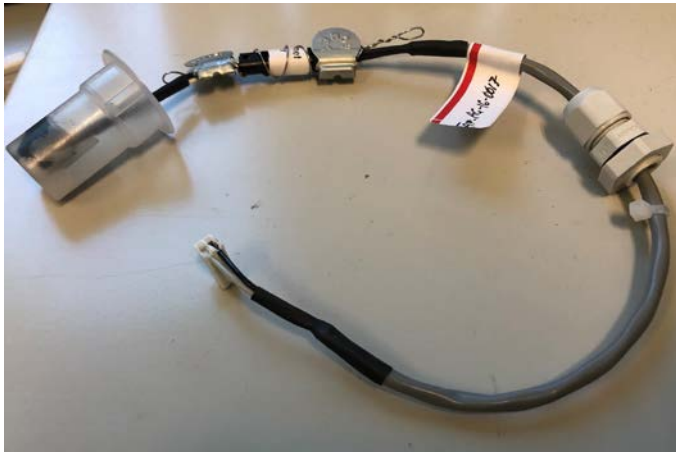
Figure 4 & 5: Typical sealing of the interchangeable Wiegand sensor assembly / Scellage typique de l'ensemble capteur Wiegand interchangeable.
