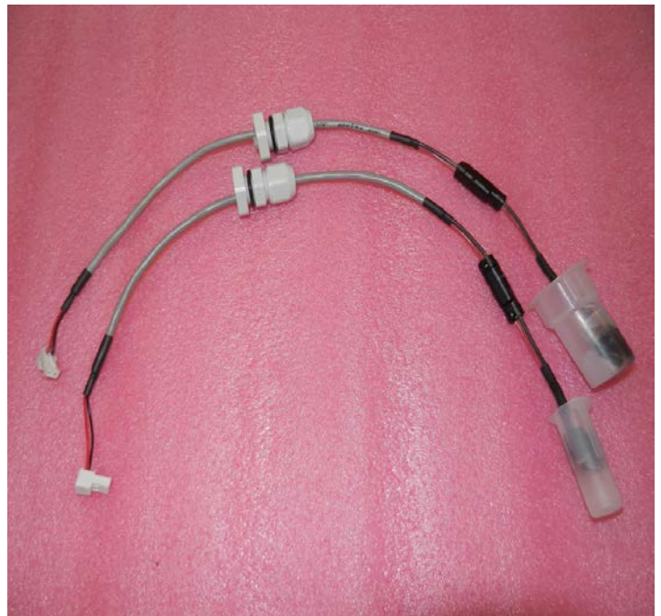
Figure 3: New AdEM Wiegand sensor assemblies.
