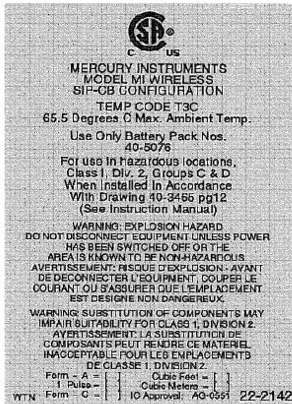
Note: This label shall be used on the outside of the instrument. A clear overlay is applied over the markings at the bottom portion of the label after marking the applicable boxes.
