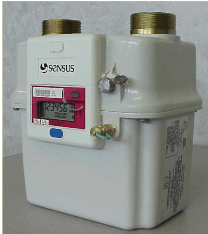
Fig. 1 : Sealing Provisions/Configuration de scellage
