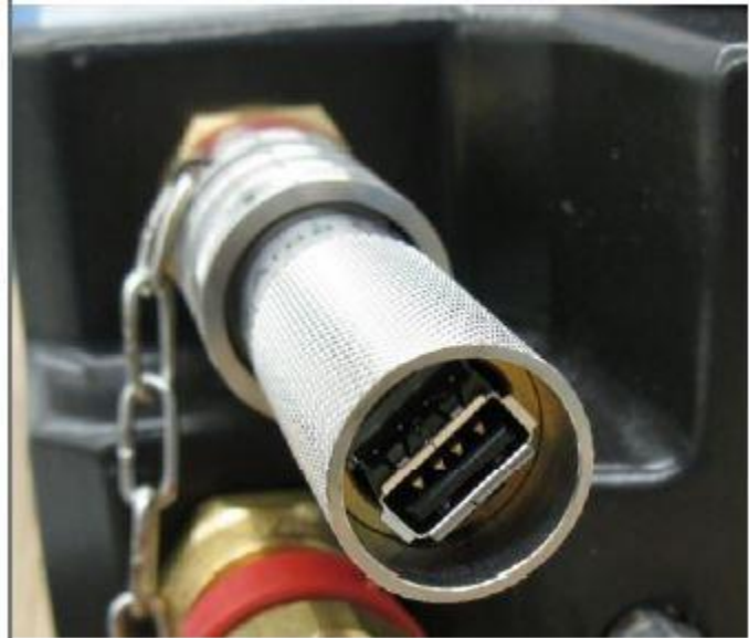
Figure 3. Optional USB port / Port USB en option
