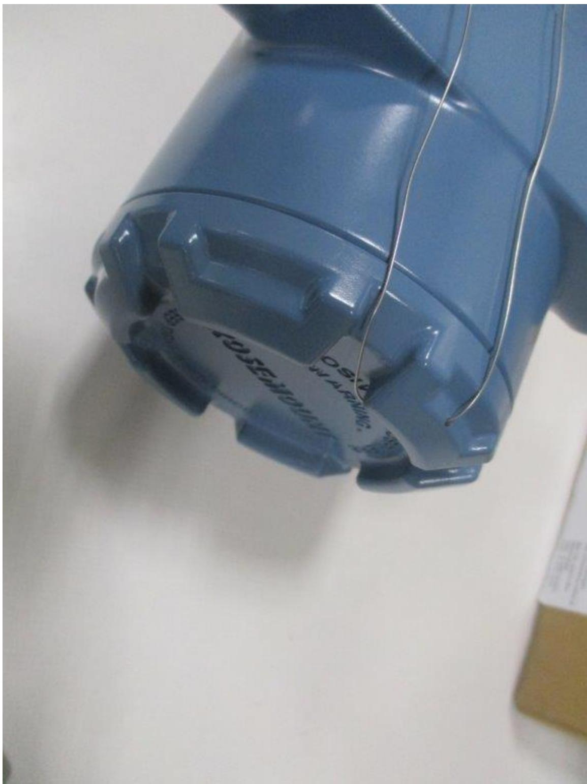
Figure 3: Sealing of housing / Scellage du boîtier
