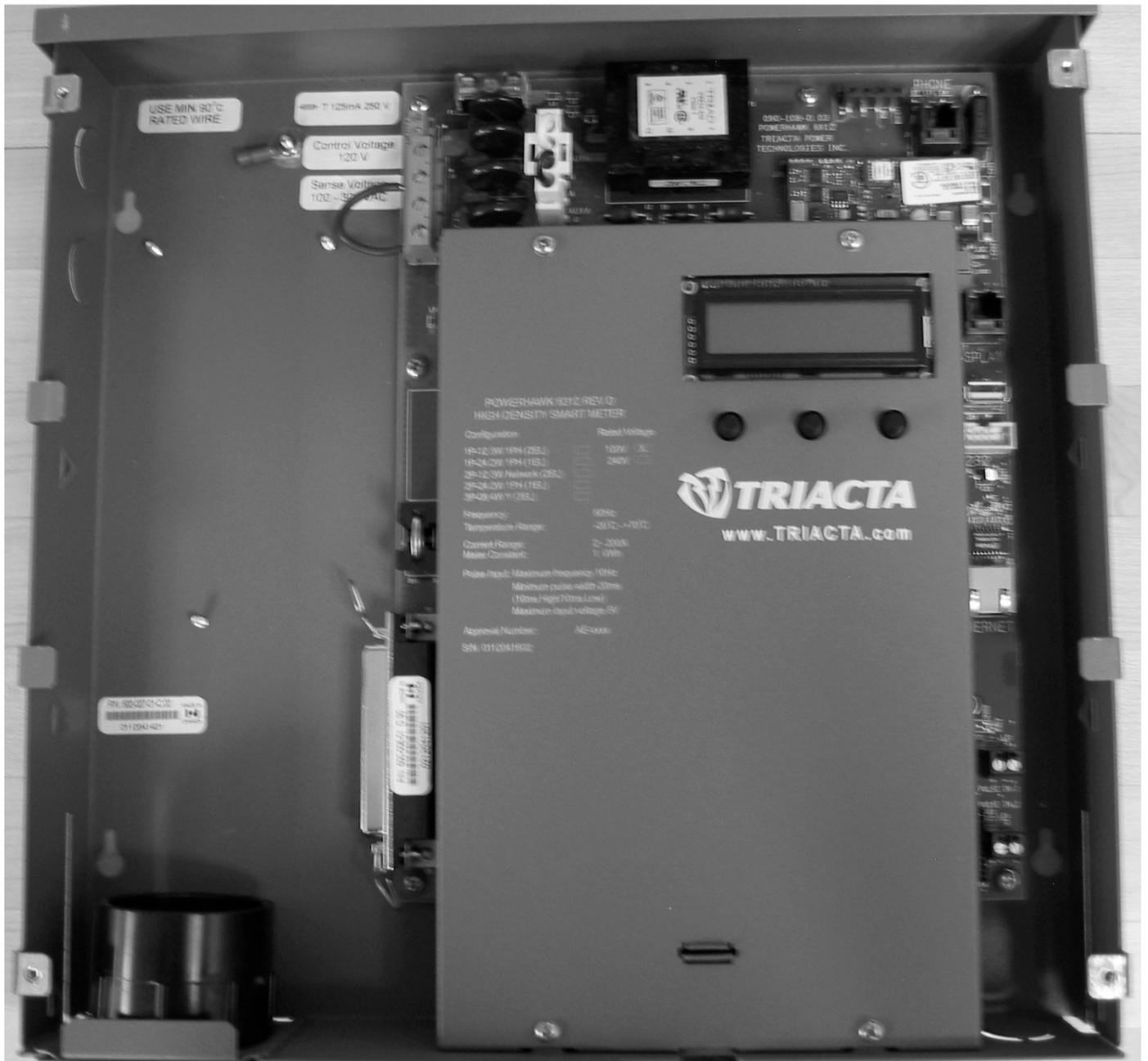
**Fig. 2 :** PowerHawk 6312 Rev. D (outer cover removed)/
