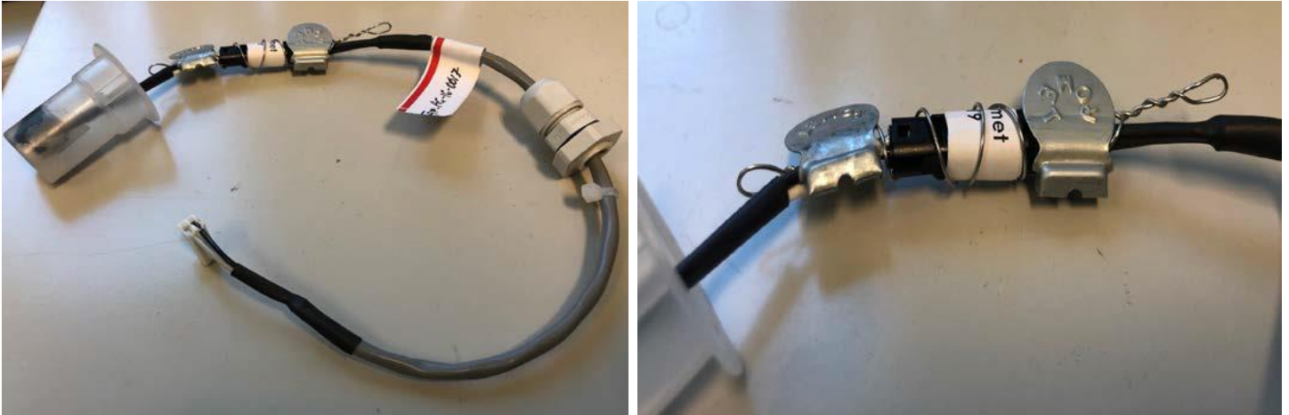
Figure 20: Typical sealing of the interchangeable Wiegand sensor assembly / Scellage typique de l'ensemble capteur Wiegand interchangeable
