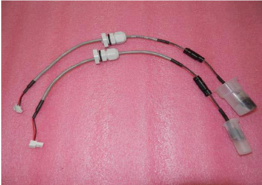
**Figure 16:** 46-124-10/46-124-20 (top) and 46-124-10/49-124-20 (bottom) wiegand sensor assemblies /
