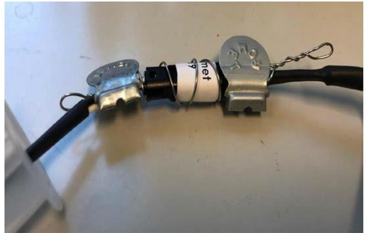
**Figure 17:** Typical sealing of the interchangeable Wiegand sensor assembly / Scellage typique de
