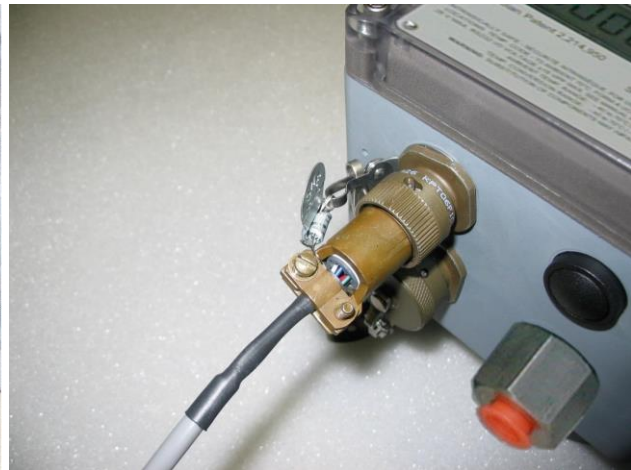
Figure 7: Wire seal on AdEM-PTZ electronic compartment and output pulse connector as well as wire integral seal / Fil métallique et scellé sur le compartiment électronique et sortie d'impulsion du AdEM-PTZ
