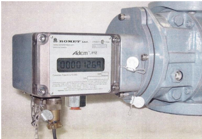
Figure 7: Wire seal on AdEM-PTZ electronic compartment and output pulse connector as well as wire integral seal / Fil métallique et scellé sur le compartiment électronique et sortie d'impulsion du AdEM-PTZ
