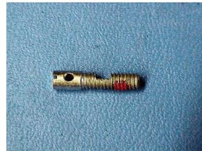
**Figure 2.** Sealing Bolt /Boulon de scellage
