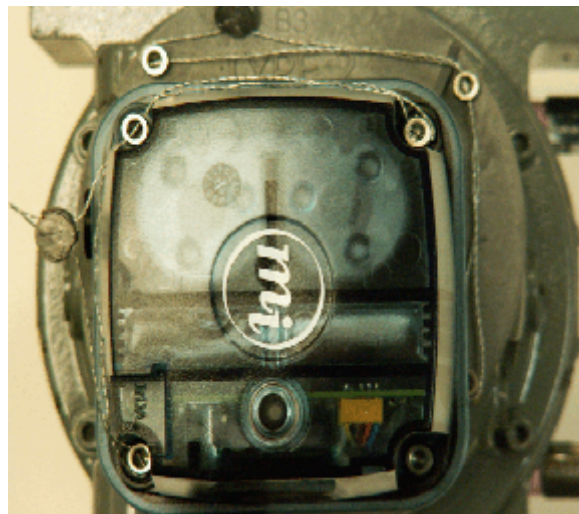
Figure 2. Sealing the TCI to the adapter plate / Scellage de le TCI à la plaque d'adaptation
