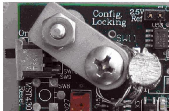
**Figure 3.** Configuration Lock Switch /
