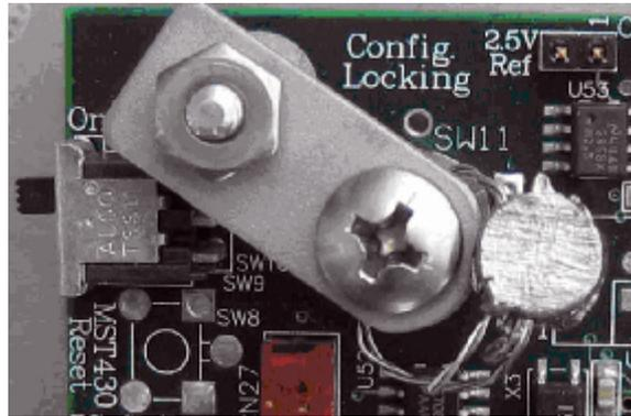
**Figure 3.** Configuration Lock Switch /
