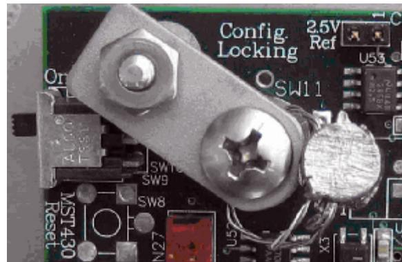
**Figure 3.** Configuration Lock Switch /
