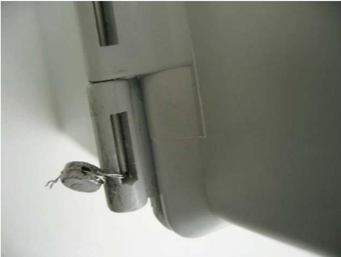
**Figure 4.** 1141C Hinge Pin Sealing /
