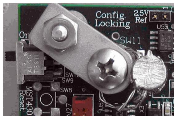
**Figure 3.** Configuration Lock Switch /
