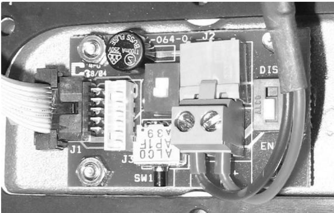
**Program (SW2), Battery Reset (SW1) and Flash Memory Program (SW3) Switches /
