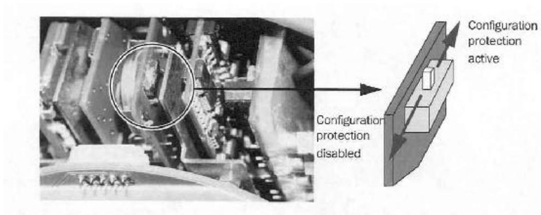
**Fig. 3: Configuration Protection Switch (Version 2 SPU) /
