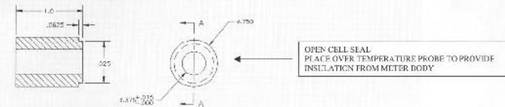
**Figure 5: ROOTS B3 Series Temperature Compensating Unit /
