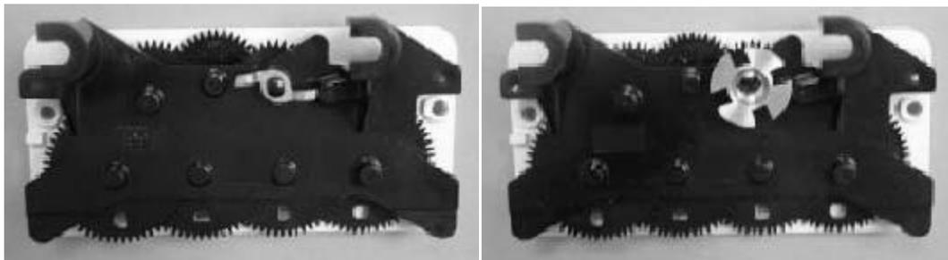
**Fig. 11:** Index with old dog / index with new dog
