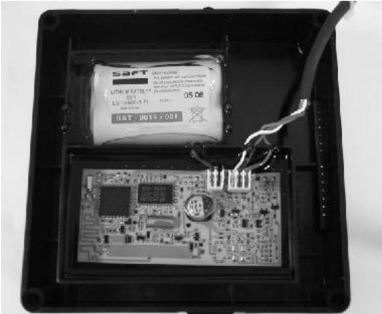
**Figure 7: 40G REMOTE ERT for connection to Mercury Conversion Devices/
