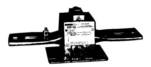
Primary input is a permanent bar of aluminum tin-plated by zincate process for 200-5 and 400-5 ratios or tin-plate copper for the 600-5 and 800-5 ratios.
