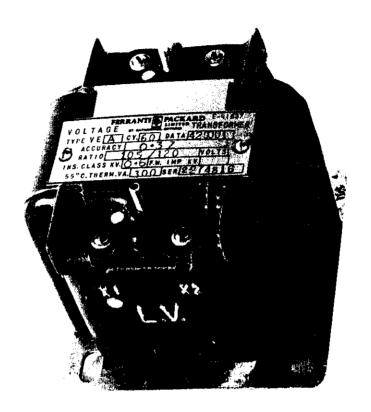
These transformers will be used with certain Type DS 15 Metering Outfits owned by Hydro Quebec to produce 120 volts from the voltage transformers rated at 13860Y/8000-100 volts to get an overall voltage ratio of 70:1. The DS 15 Metering Outfits are covered by NRC 72.
