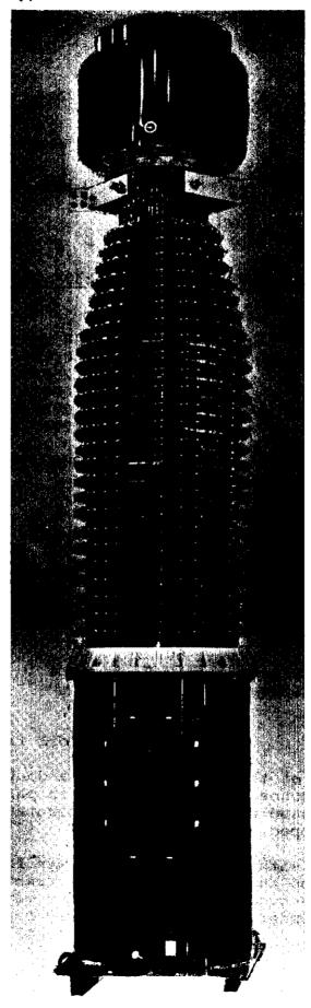
Each secondary in a multi-secondary unit is complete with its own winding and magnetic circuit and is therefore completely independent of the other(s). Its accuracy would be maintained regardless of the burden on the others(s). Because of this, any unused secondary should be short-circuited, preferably over the whole winding.
