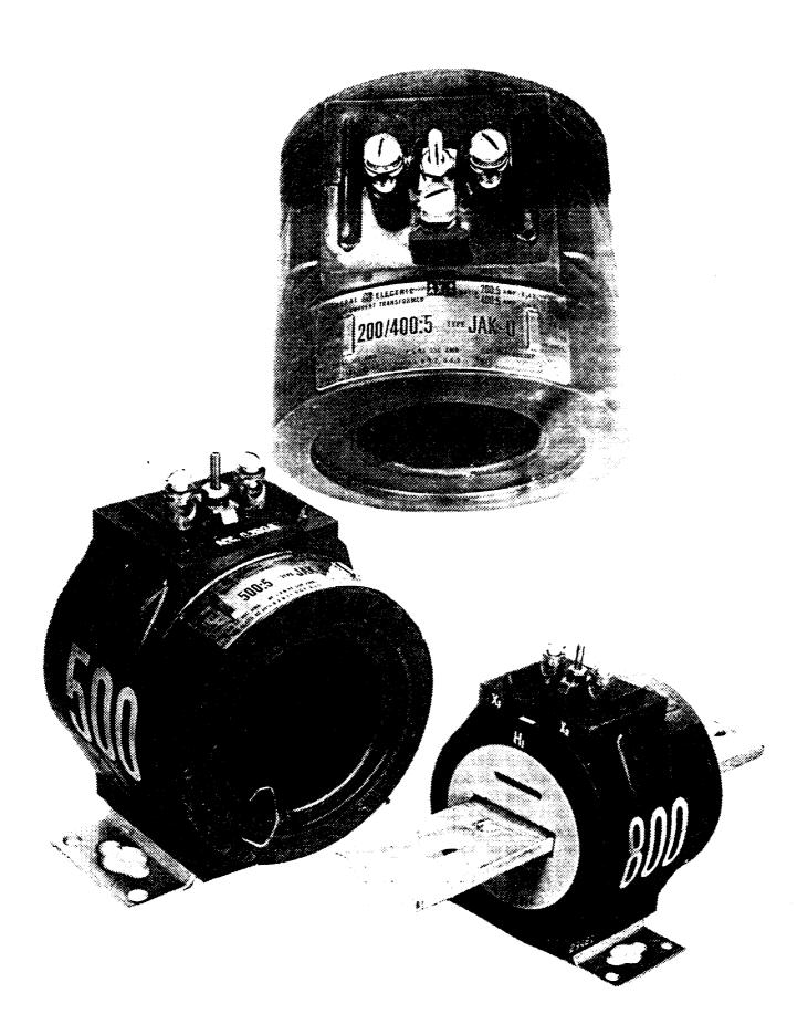
Secondary terminals are bronze stude set in the moulding on the top of the transformer and held in place by an internal terminal block. This block also secures a stude located between the terminals, which is used as the short-circuit device pivot and as a means to attach and secure the secondary cover which has an interlock to hold the short-circuit device in the open position when the transformer is connected in the operating position.
