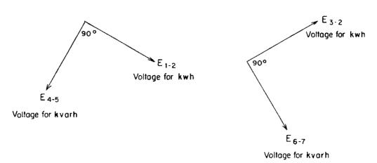
METER POT COIL "A" METER POT COIL "B"
