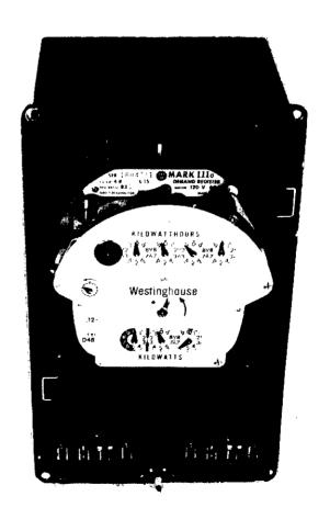
The base speed of the "D" line meters on which these registers are used is either 1000 r.p.h. or 500 r.p.h., and the disk shaft has a single lead worm that meshes with a 100 tooth pinion.
