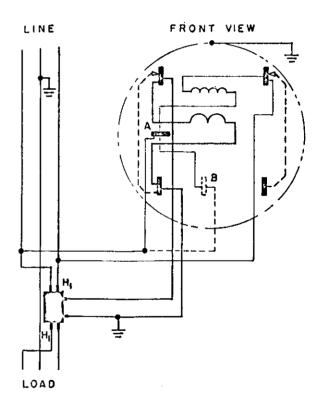
S-base, 2-wire, 0.12-10 A meter with 3-wire double-primary CT; 5-jaw socket with circuit-closing devices.
