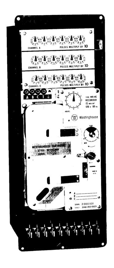
They record on magnetic tape (a) pulses proportional to the load being metered and (b) time interval pulses. The tape is the same in all cases, but the type "WR-2C" has in addition to the time pulse track, only a single track for load information and the type "WR-4C" has three such tracks.
