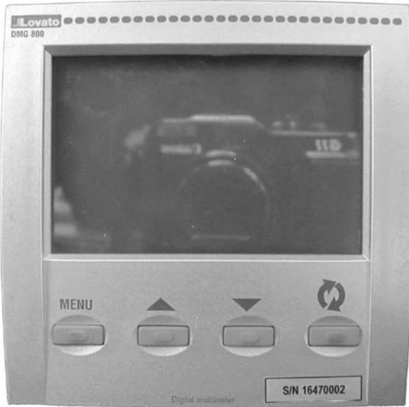
**Figure 4: Meter face with auxiliary serial number nameplate /
