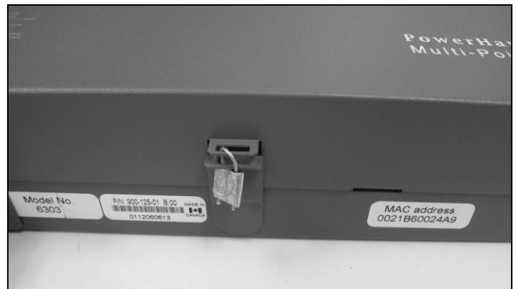
Installation Sealing Location / Emplacement du sceau du service public.
