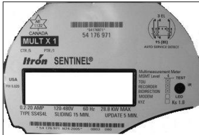
Nameplate with Trilliant Networks NCZR801PH-SENT / Plaque signalétique avec Trilliant Networks NCZR801PH-SENT
