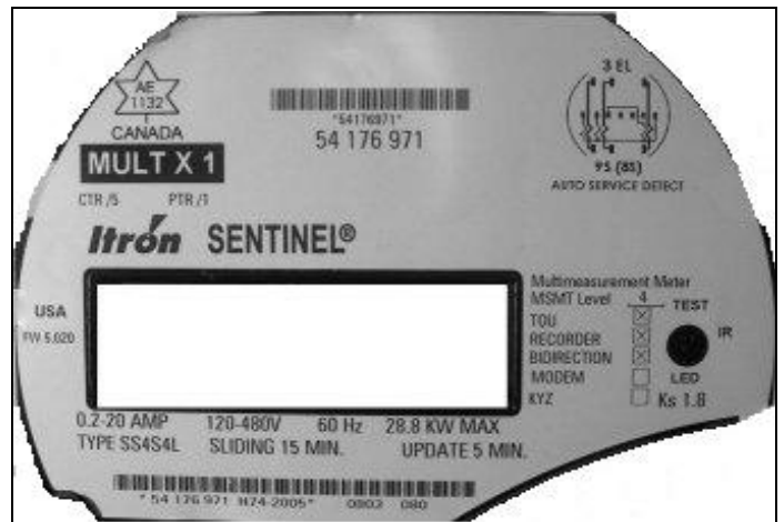
Rev. 11 Sentinel with Trilliant Networks NCZR801PH-Sent SecureMesh™ module nameplate / Rév. 11 Plaque de Sentinel avec module NCZR801PH-Sent SecureMesh™ de Trilliant Networks
