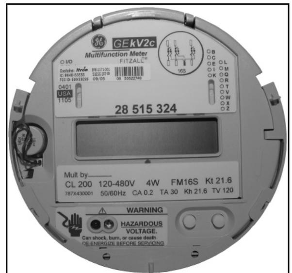
**KV2c retrofitted with 53ESS Itron
