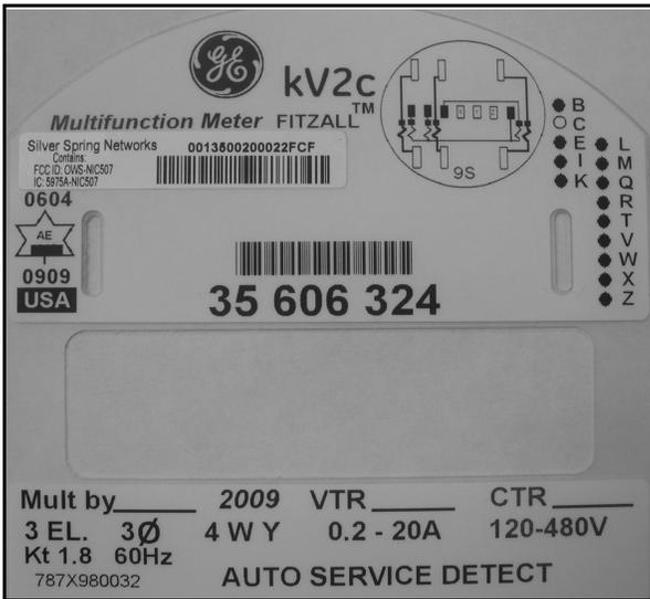
kv2c markings with new SSN module /
