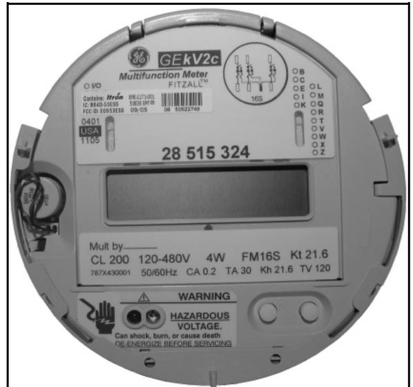
**KV2c retrofitted with 53ESS Itron module/
