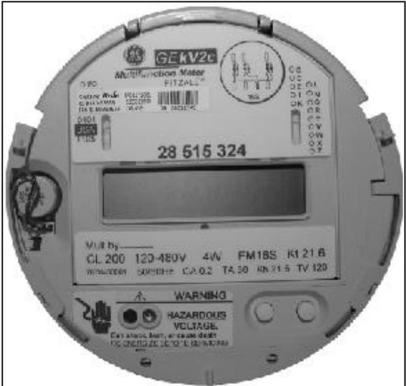
**KV2c retrofitted with 53ESS Itron module/
