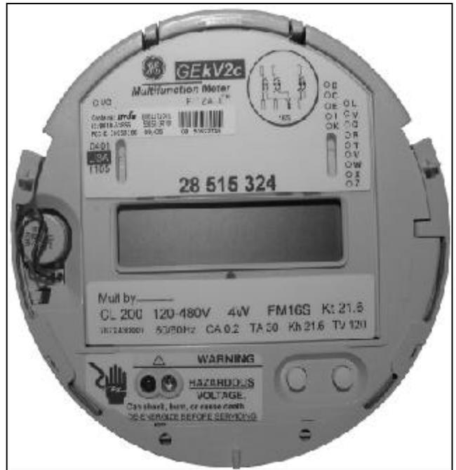
**KV2c retrofitted with 53ESS Itron module/
